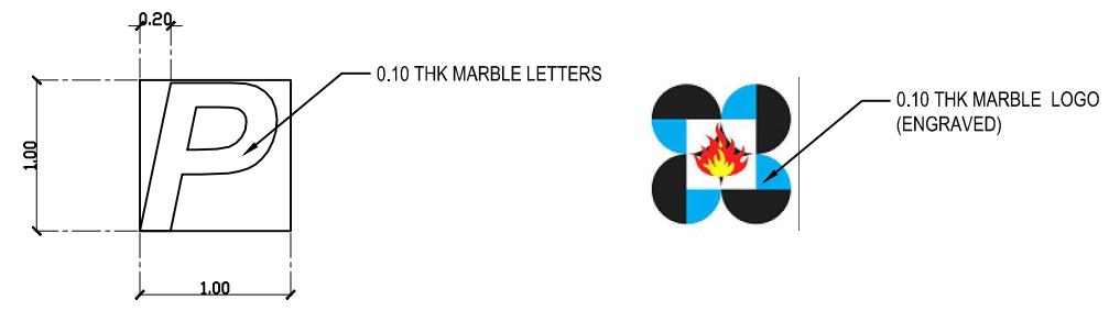
PHILIPPINE SCIENCE HIGH SCHOOL - MIMAROPA REGION CAMPUS MARBLE LOGO AND LETTERS SCALE: 1:4
